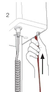
The electrical emergency lowering device feeds out the lift strap for as long as the emergency stop strap is held down. Ensure that the lowering motion is activated. Otherwise, electrical emergency lowering must be stopped. Always ensure that emergency lowering is done in an appropriate location.
